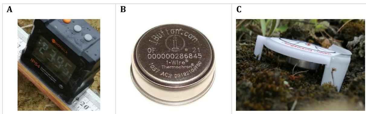
FIGURE 13 : (A) CLINOMÈTRE ; (B) THERMOCHRON ; (C) THERMOCHRON SOUS UNE ENTRETOISE.
